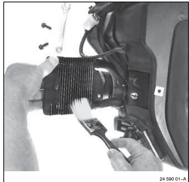
Figure 2-5 Cleaning the Oil Cooler
